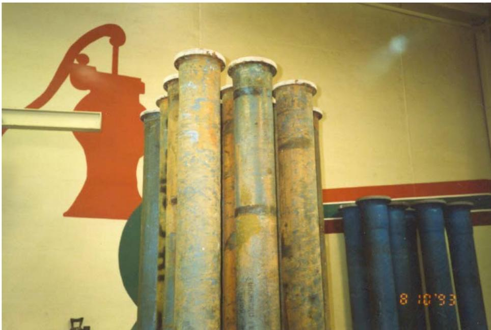
**Figure 6. Sections of FIBERBOND(R) column pipe after ten years service, next to new sections of FIBERBOND(R) column pipe. There is no structural material loss on the ten-year old column pipe; only a slight "scale" buildup on the exterior. In some places, the gelcoat exterior (blue) is still intact.**
