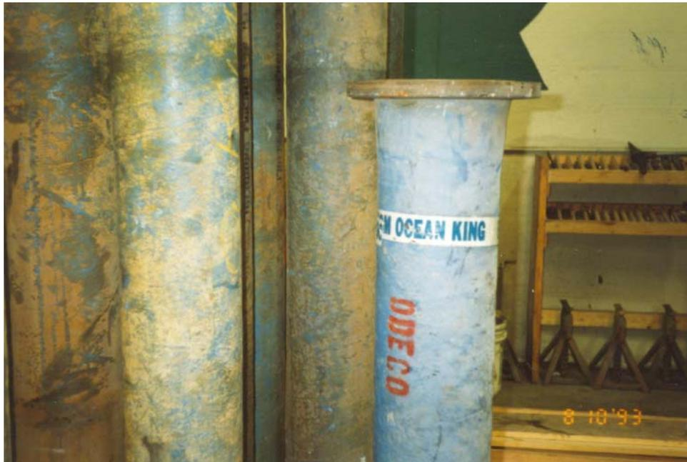
**Figure 5. FIBERBOND(R) column pipe in shop for inspection after ten years service in the Gulf of Mexico. Steel column pipe would last an average of three years under same conditions.**
